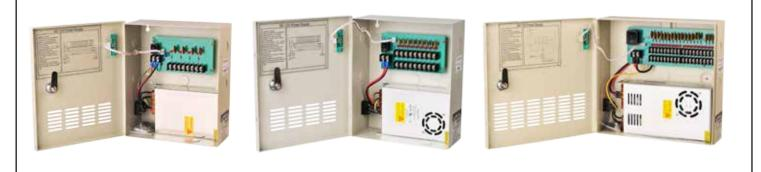
The power distribution system of metal boxed power supply makes it with multiple outputs, Individual PTC resettable fuses on channel boards can protect the device from over load or short circuit. Output voltage is adjustable to bear voltage drop after longer distance transmission. The device is your first choice of power solution in CCTV System.
